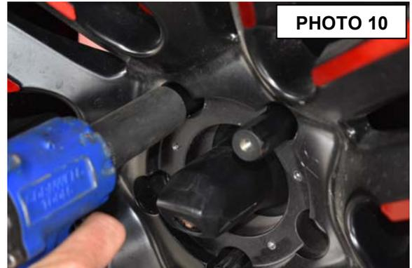
10. Install the supplied 3rd brake light bracket using the (2) supplied 8mm x 25mm bolts (70055BAG1) onto the (2) upper supplied lug nuts. **See Photo 11.**
