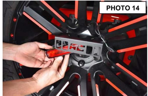
14. Using the factory screws, secure the 3rd brake light to the bracket and carefully tighten using a T25. **See Photo 15.**
