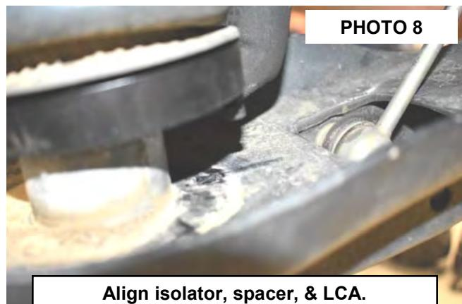
11. Once all components are properly aligned, use a jack to raise the lower control arm and install the factory lower control arm bolt. **See Photos 9 & 10.**
