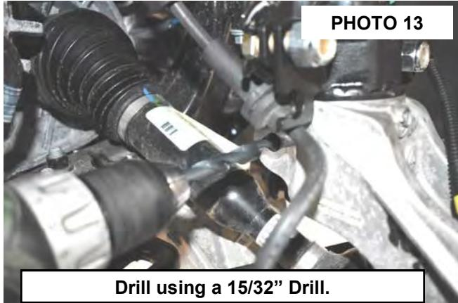
Drill using a 15/32" Drill.
