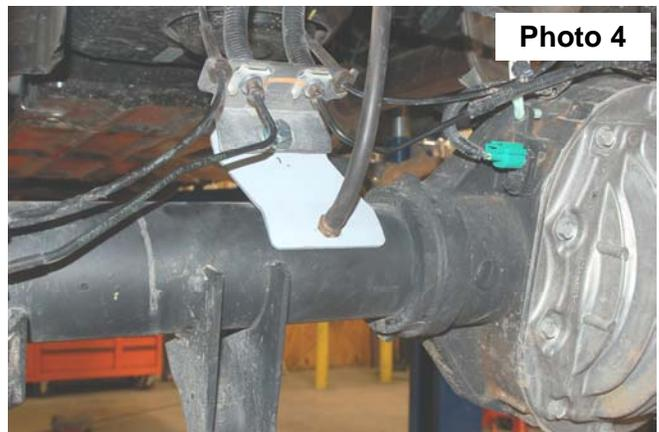
7. Using a 24mm socket, remove the stock u-bolts. Use the floor jack to lower the axle assembly to allow for lifted block installation.
