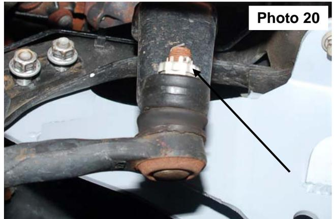
38. Dislodge link with a tie rod end puller, or a pickle fork. Note: replace the link if any stud looseness is detected, or if you can twist the studs in its socket with your fingers.
