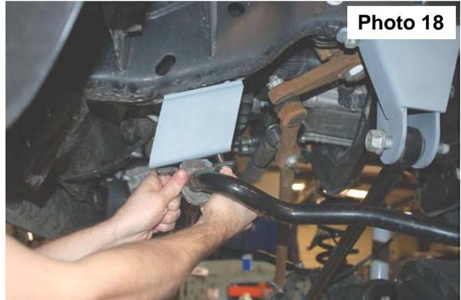
36. Install the stabilizer in the bracket using the stock hardware. **See Photo 19.**
