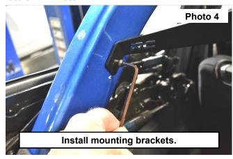
3. Install the sound bar to the Dr/Pass side mounting brackets with the hardware supplied with the soundbar. See Photo 5 and Photo 6.
