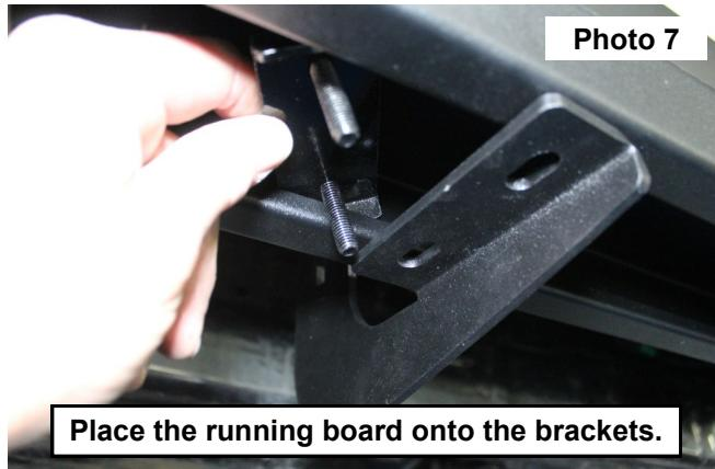
Place the running board onto the brackets.
