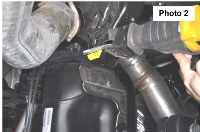
9. Install the new supplied track bar bracket with the crush sleeve using the supplied 9/16" x 4.5" bolt, washers, and nut. Hand tighten. Use the bracket as a template and drill the hole using a 17/32" drill bit. Next install the 1/2" x 1.5" Grade 8 bolt and nut in the drilled hole. Torque the 9/16" bolt to 130ft/lbs with a 13/16" socket & wrench and torque the 1/2" bolt to 90ft/lbs with a 3/4" socket and wrench. **See Photo 3.**
