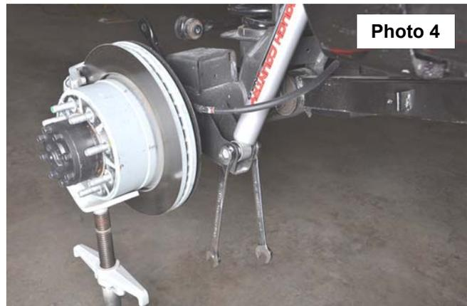
11. Next install the rear sway bar links using the supplied 12mm x 75mm bolts, lock nuts, and washers. Torque to 75ft/lbs with a 18mm and 19mm wrench.
