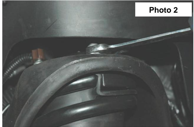
5. Place jack stand under the knuckle for support. Remove upper ball joint nut, using a 18mm wrench. Using a hammer hit the knuckle as shown to allow the ball joint to separate from the knuckle. **See Photo 3.** Do not allow the knuckle to pull out far enough that it pulls the shaft out of the differential.
