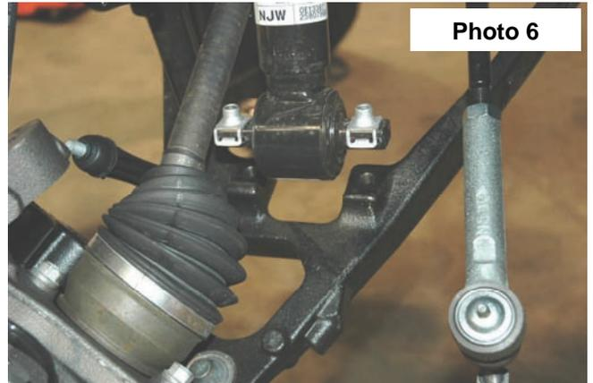
9. Remove the bolt clips from the bottom of the strut using a flat screw driver. **See Photo 7.**
