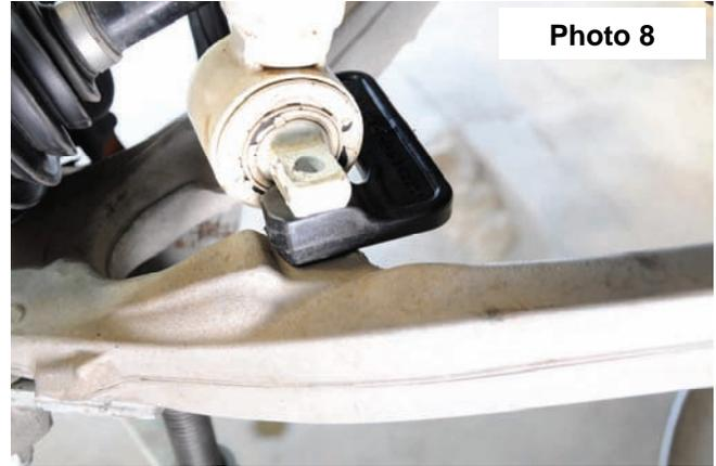
11. Install the new 10mm bolts, washers and nuts provided in the kit. . Install bolts with the head going down as shown in **Photo 9.** Tighten to 30-35 ft/lbs. **Do not over-tighten the bolts.** You may have to move the knuckle to one side to allow room to install the bolt by the axle shaft.
