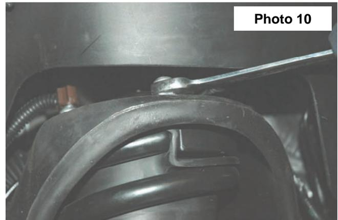
14. Raise the lower control arm and connect the upper ball joint on the upper control arm to the spindle. Using a 18mm wrench, torque to manufacturer specs. If ball joint turns while tightening, use a 7/32" allen wrench to hold the ball joint. **See Photo 11.**
