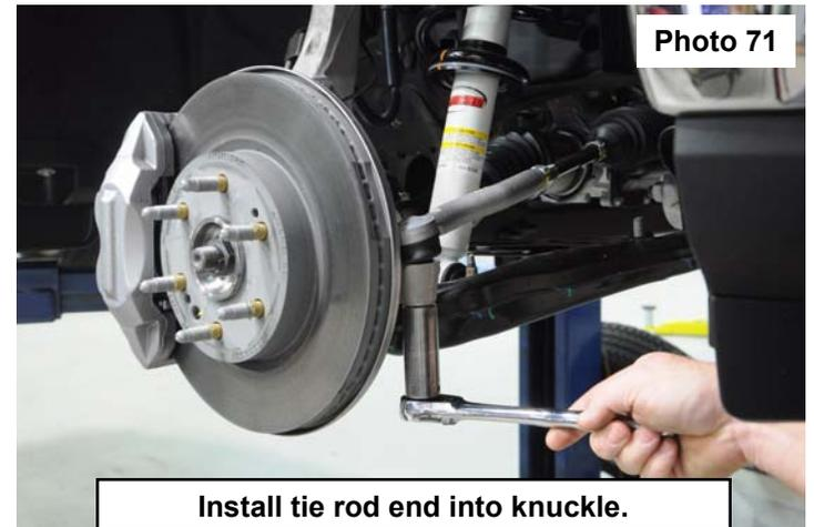
Install tie rod end into knuckle.
