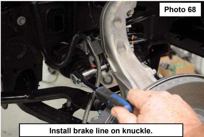
Install brake line on knuckle.
