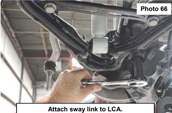
Attach sway link to LCA.
