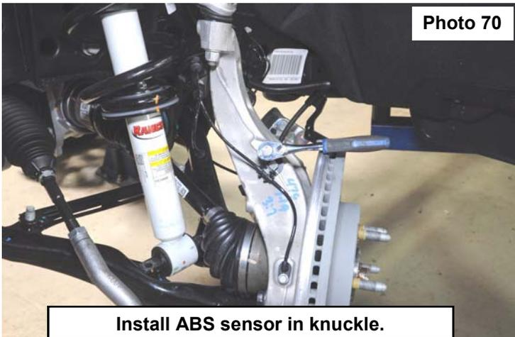
Install ABS sensor in knuckle.
