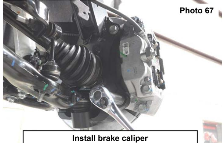
Install brake caliper
