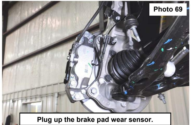
Plug up the brake pad wear sensor.
