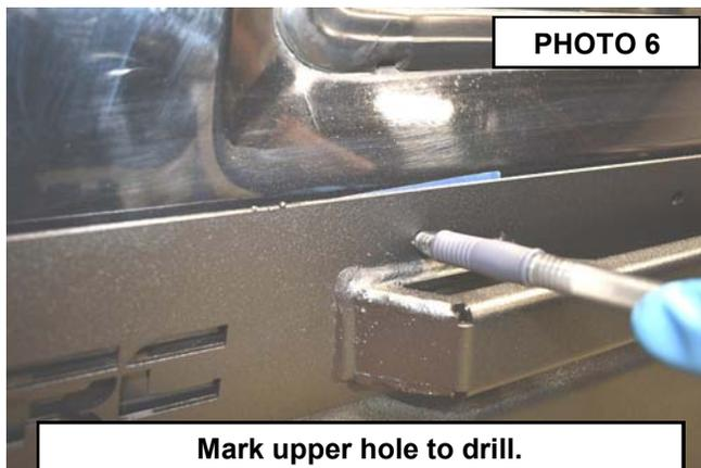
12. Remove the panel and drill **ONE** of the holes using a 1/4" drill bit. Realign the panel by placing a provided 1/4-20 x 3/4" through the hole and threading the nylock nut and washer onto the back. **See Photo 7.**
