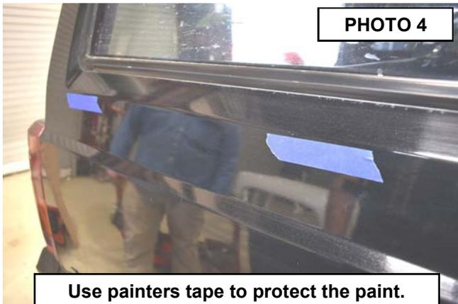
10. Start with the rear driver side panel. This will be the hardest to install because of the spare tire bracing and fuel filler neck.
