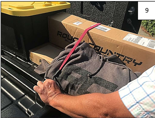
Use bungee cords (not provided) to secure items being stored in tray. Insert hooks through slots around perimeter of Bed Storage Tray. Criss Cross bungee cords to secure items.
