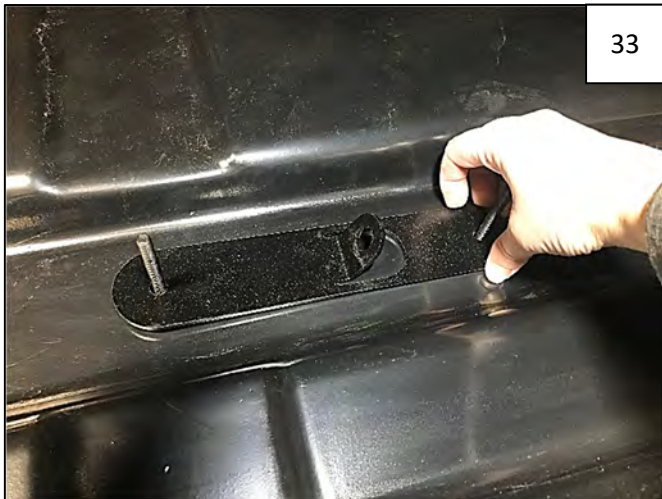
Install a supplied Inner Tie Down Bracket over the threaded bolts, from the inside of the Box.
