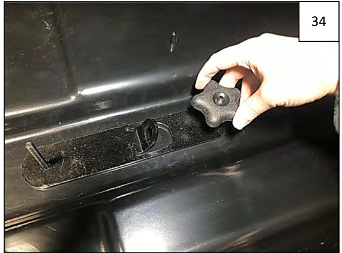
Place a Plastic Knob over each threaded bolt and tighten down to secure Bar Clamp and Inner Tie Down Bracket.
