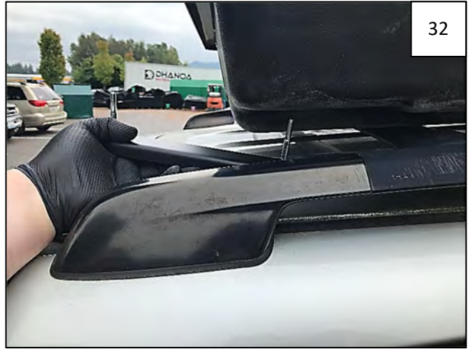
Slide a supplied Bar Clamp underneath roof rack cross bar and up into box, capturing the cross bar. Insert two threaded bolts on Bar Clamp up through nearest holes in part.
