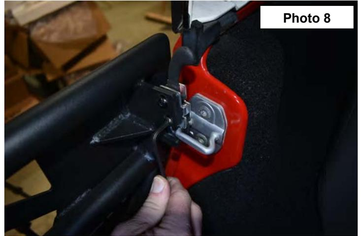
9. Check to see if a shim is needed on the latch mechanism by closing the door. Shim latch as needed to engage the door pin and tighten using a 4mm Allen wrench. **See Photo 9.**
