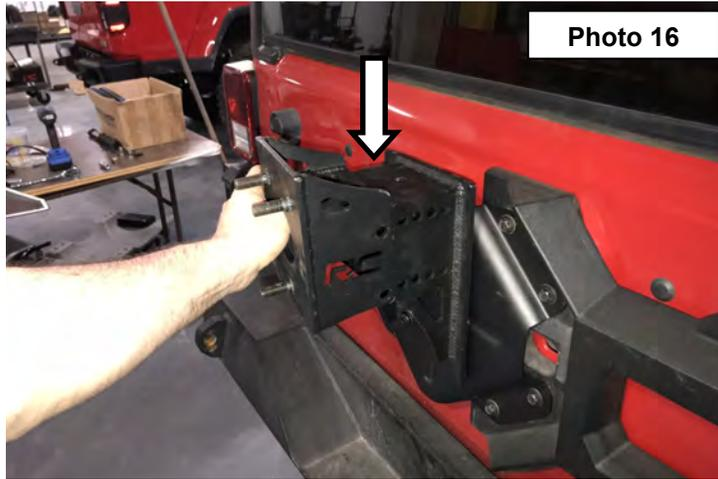
15. Secure with the (4) 10mm x 30mm Button head bolt, flat washers and (4) 10mm lock nut. **Photo 17.** Install the tire and wheel with one lug nut, adjust as needed and mark optimum location. Remove the tire/wheel from mount and tighten bolts using a 14mm wrench and 6mm allen wrench.
