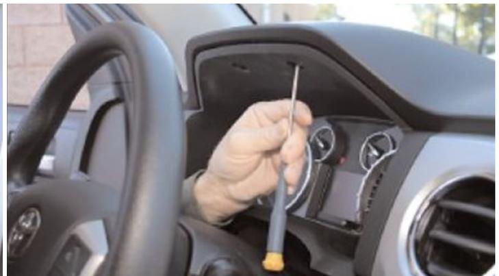
10. Once you push in the center of the retaining clips they can be removed and then the trim piece can be removed.
