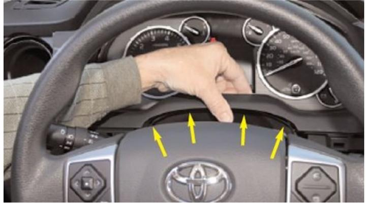
12. Using an 8mm socket remove the four (4) retaining screws and pull out on the IPC.
