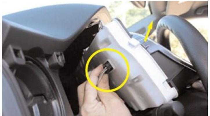
14. Connect the male end of the Speedometer Calibrator Harness to the factory wiring harness and the female end into the Instrument Panel Cluster.
