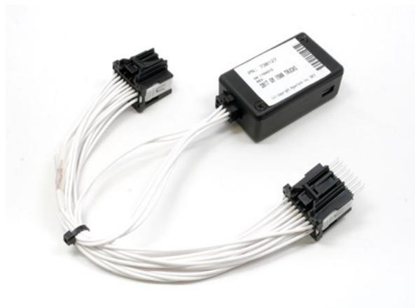
2. There is a small module with 2 connectors, underneath the dash on the left side, above the emergency brake pedal. This will be in front of a larger module with several connectors. We will be removing the black connector. With a pick or small screwdriver, slide the red locking clip backwards and depress the tab on top while pulling back to remove the connector.
