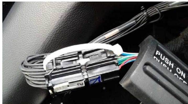
4. Connect the female end of the Speedometer Calibrator harness into the vehicle's module.
