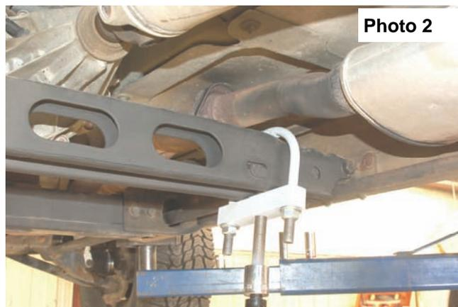
Reinstall the threaded block and adjuster bolt.
