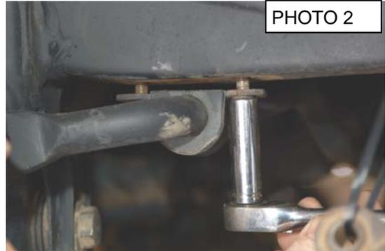
6. Remove the cotter pin on the tie rod and remove nut using a 19mm wrench. Strike the end of the knuckle to dislodge the tie rod. Retain the hardware for reuse
