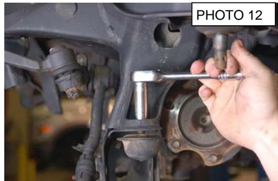
15. Remove the two factory bump-stops from the frame using a 14mm wrench as shown in **Photo 12 & 13**.
