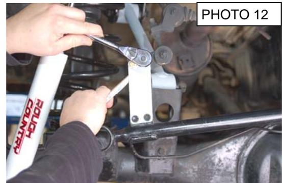
19. Install the bracket on the track rod with factory hardware using a 12mm wrench. Install the stock bracket on new bracket with the supplied 5/16" x 1" bolts using a 13mm wrench. **See Photo 12.**
