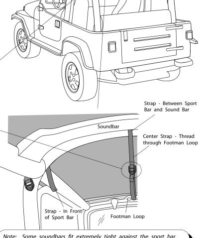
Note: Some soundbars fit extremely tight against the sport bar preventing the buckles easy access to the straps. If this is the case, the soundbar must be moved slightly rearward. The distance will vary on each vehicle.
