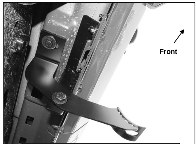
(Fig 6) Driver/left front Brackets installed
