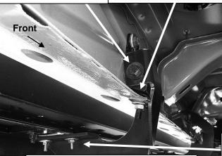
(Fig 24) Passenger/right side front Bracket attached to Running Board
