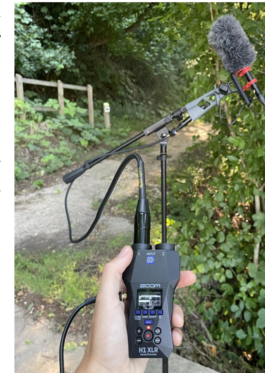
Figure 2. Rodent NTG5 Shot-Gun Microphone connected to a ZOOM H1 XLR Handy Recorder outputting into a standard pair of headphones.
