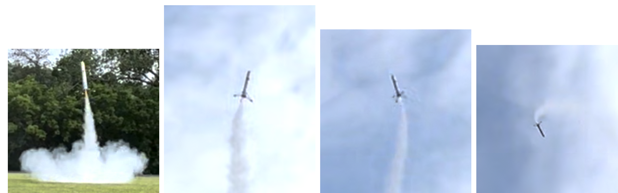
Figure 3. TMV reacting to the deviation detected by the IMU sensor onboard, last picture shows an over-correction of TVM
