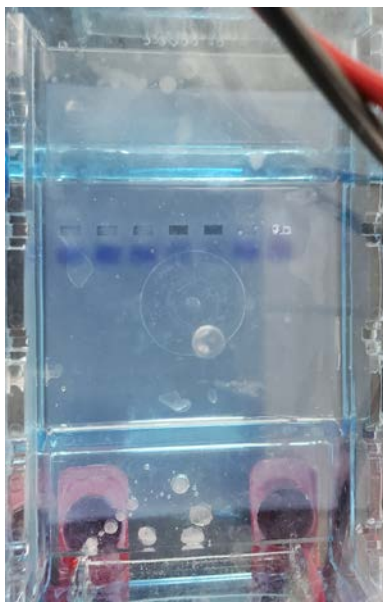
Figure 4. Agarose gel during electrophoresis process. Note the tracking dye (blue).
