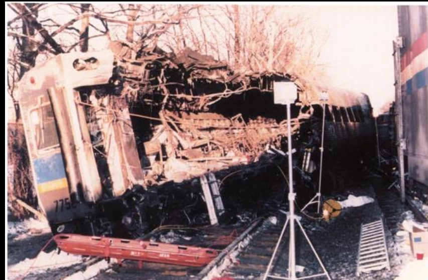
Figure 6--Photograph of postcollision passenger coach cab control car 7752 at accident site.
