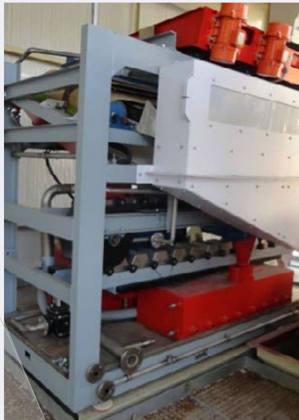
Grease belt technology is being used at OLDM to recover more diamonds
