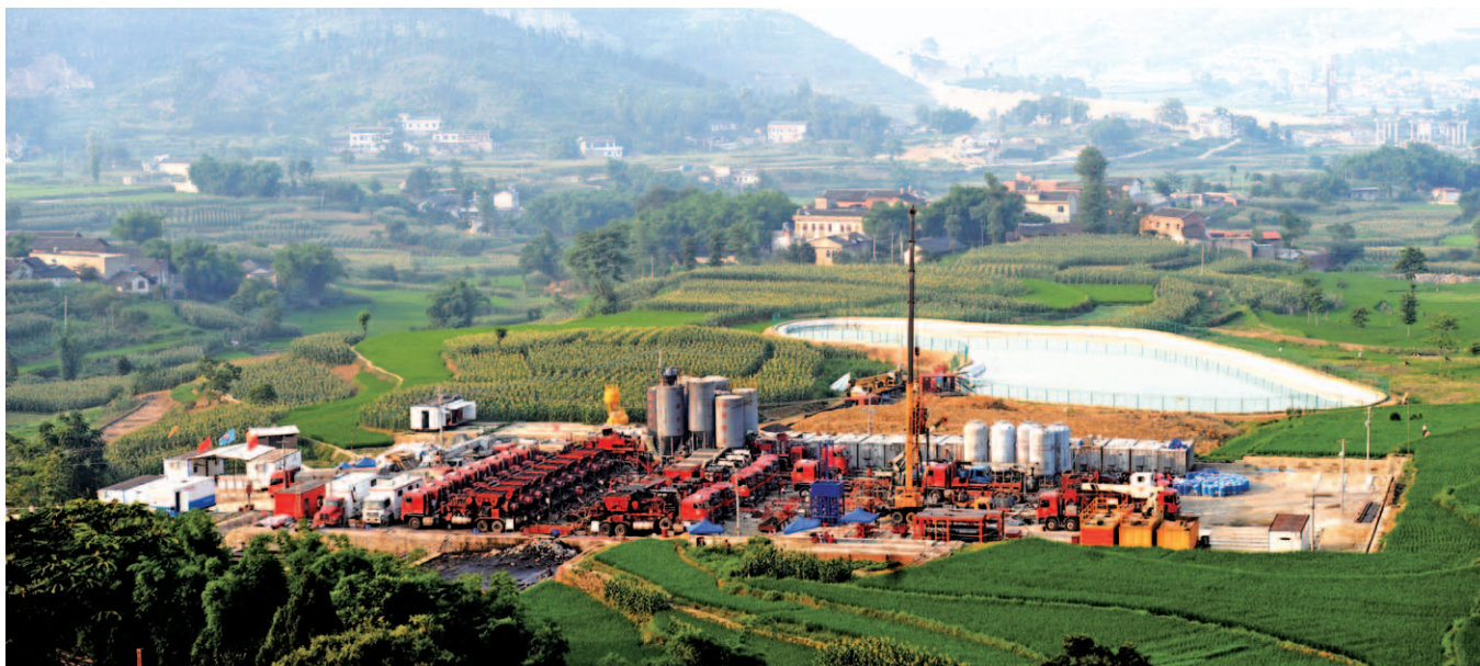
Sand fracturing operation at Weiyuan shale gas block in Sichuan
