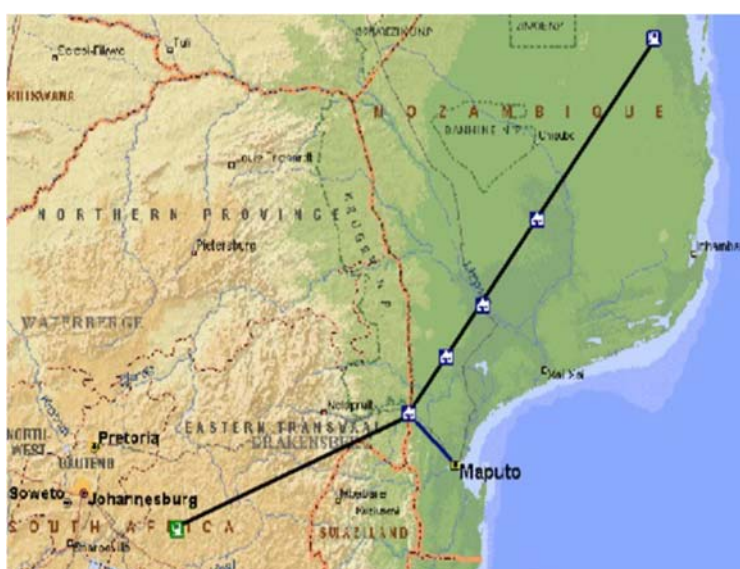
Figure 5: Route of the Temane – Secunda gas pipeline, outlet points and Maputo branch pipeline
