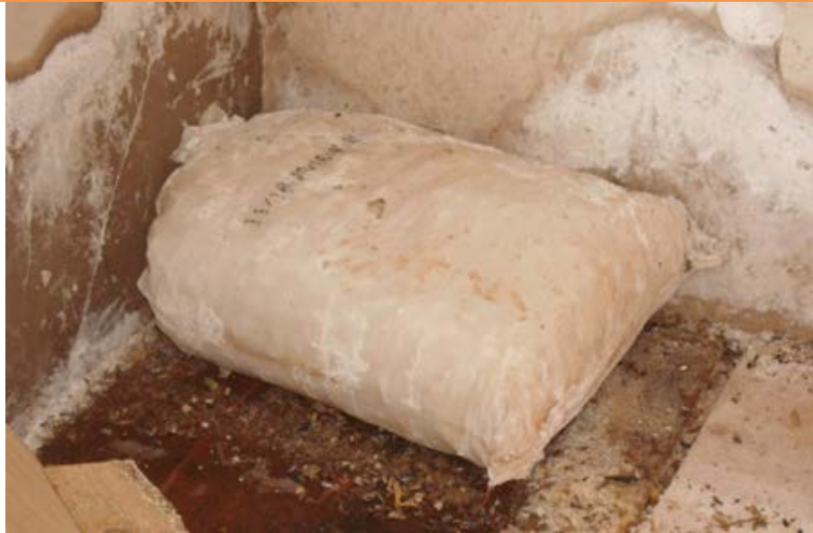
Cyanide bag placed on wet floor
