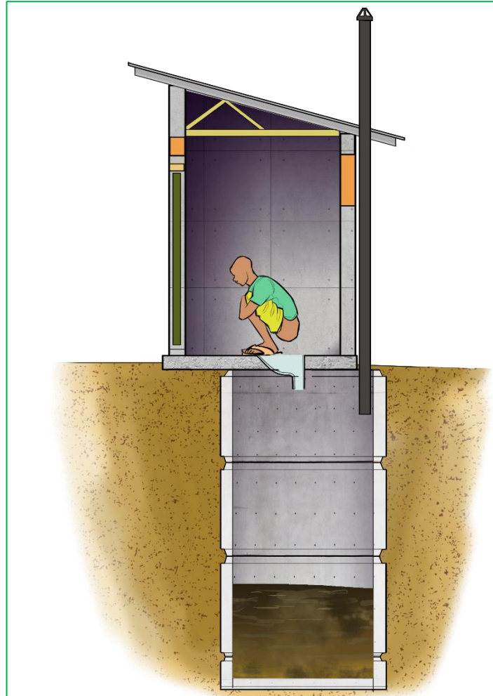
Figure 2-5: Precast Concrete VIP latrine
