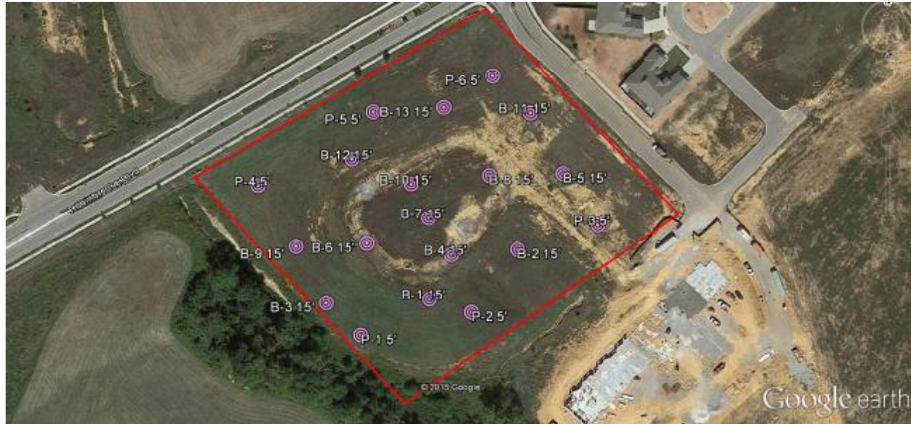
Figure 2: 2015 Google Aerial – Boring Locations Over Existing Conditions
