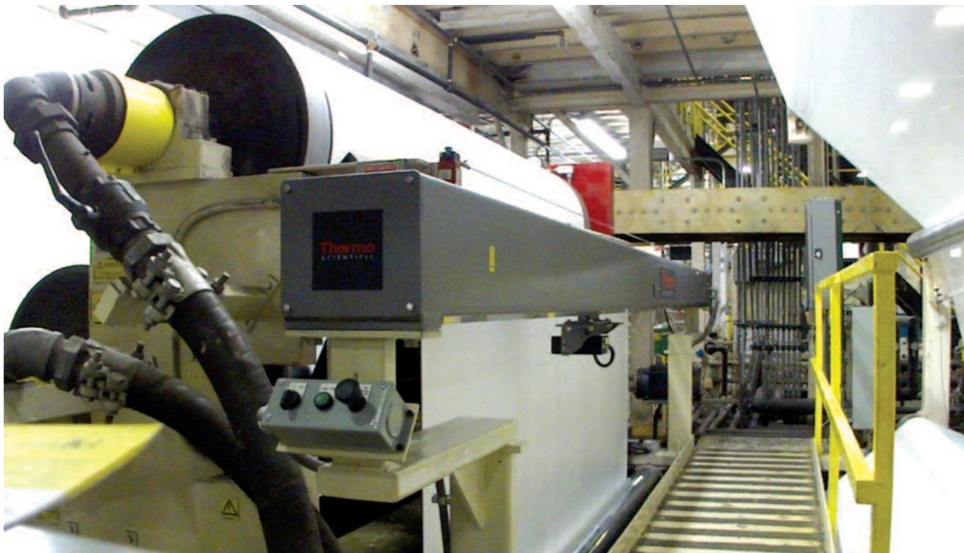
**Picometrix built the first commercial terahertz device, T-Ray 2000, in 1999 for university R&D and the first industrial terahertz device with CE UL certification, T-Ray 5000, in 2012. The T-Ray 5000 is shown here controlling layer thickness on co-ex TPO roofing.** Photo courtesy of Picometrix
