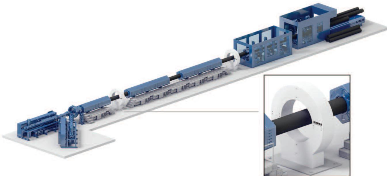
**Sikora offers a new millimeter wave thickness measuring device called Centerwave 6000 in five sizes for pipe from 90 mm to 3.2 meters in diameter. Its first millimeter device was sold in May to control wall thickness of monolayer sheet; the second will control monolayer pipe.** Photo courtesy of Sikora
