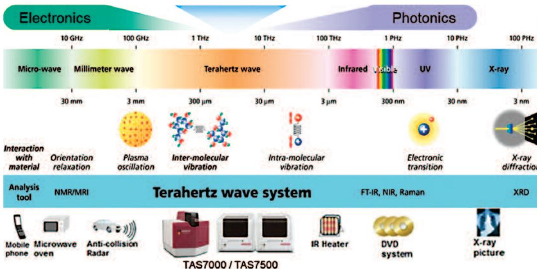
Terahertz waves reflect, pass through, or are absorbed differently by different plastics, so they can measure layers inside a plastic wall without contact. A pulsed terahertz signal returns from layered surfaces, is reflected onto a sensor, and interpreted by software to measure layer thickness.
