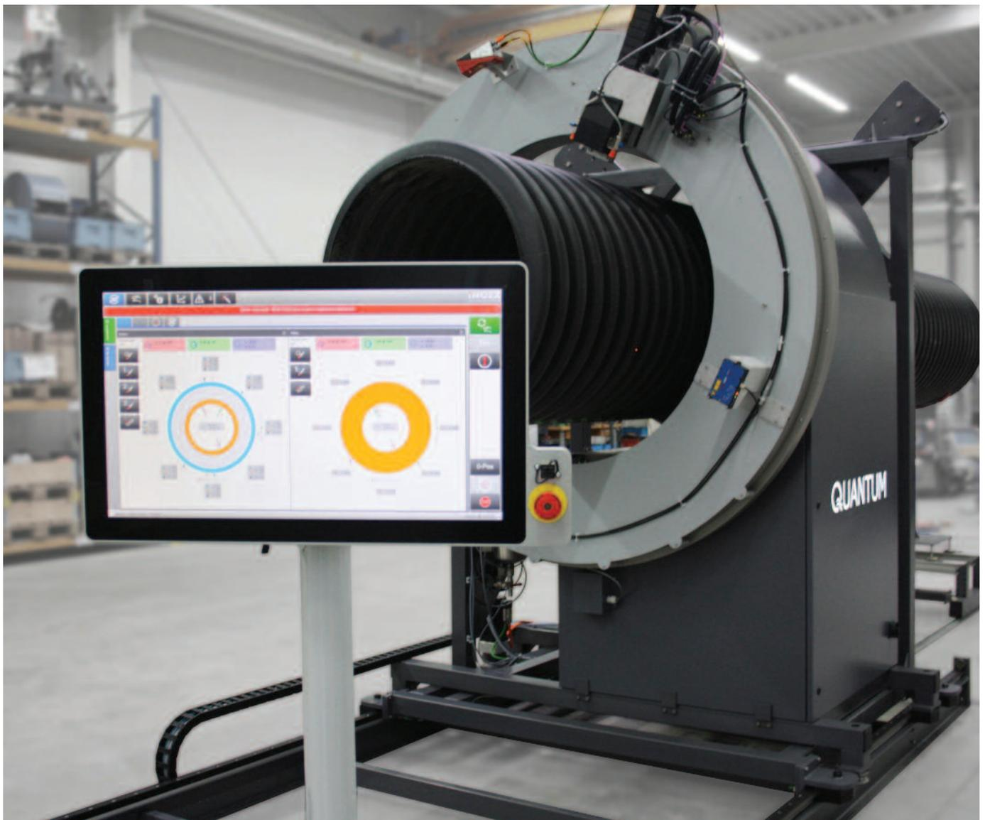
iNOEX's Quantum 360 terahertz device controls pipe wall and layer thickness in foam core PVC and corrugated pipe, which can't be measured by ultrasound gauges in water because of air in the pipe walls. Terahertz is noncontact, so devices don't need to be sized for each pipe diameter. Photo courtesy of iNOEX
