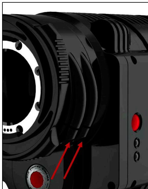
Loosening RED ONE Focus Ring Bolts
