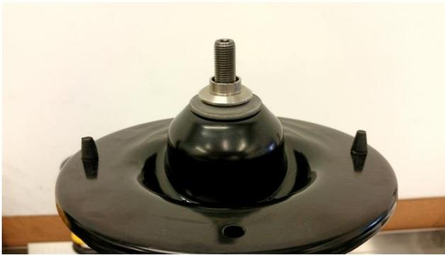
6. Place the RCE Camber Plate on top of the RCE lower spool.
