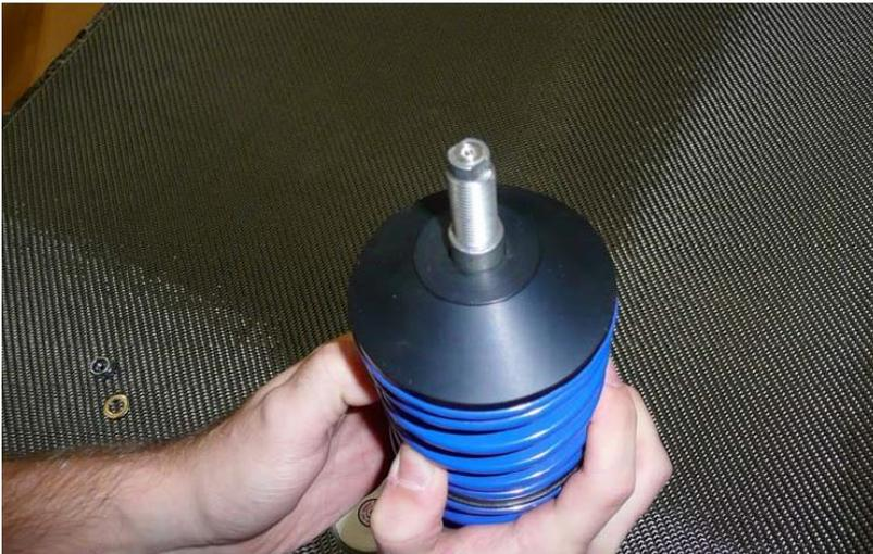
3. Install the provided RCE lower spool washer onto the top spring plate.
