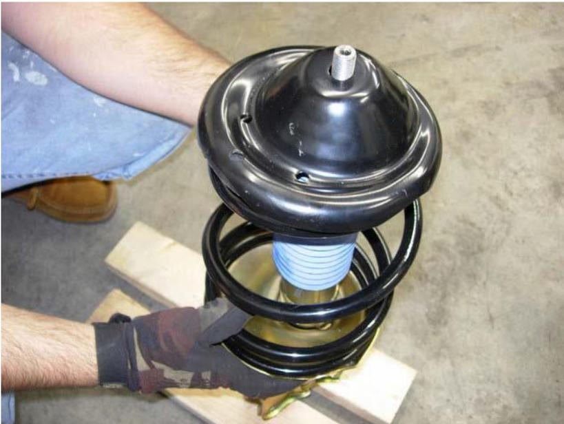
3. Align upper metal spring perch so that the three holes in the perch that form a triangle point outward towards the strut mounting tabs on the bottom of the strut.
