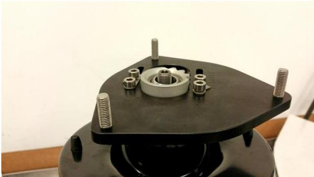
7. Carefully thread the RCE provided top nut on to the strut shaft. Torque to 40 ft-lbs.
