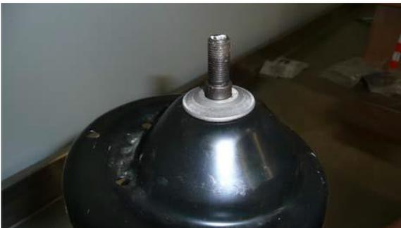
5. Place the RCE provided lower spool washer on top of the Subaru Conical washer.
