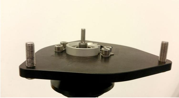
5. Carefully thread the RCE provided top nut on to the strut shaft. Torque to 40 ft-lbs.
