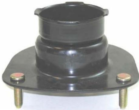
2) The mount is clearly separated into two individual steel stampings, with the bottom portion shaped like an inverted cup with 4 prongs around its perimeter. You will be cutting the mount where the two stampings are joined marked with a dotted white line here:
