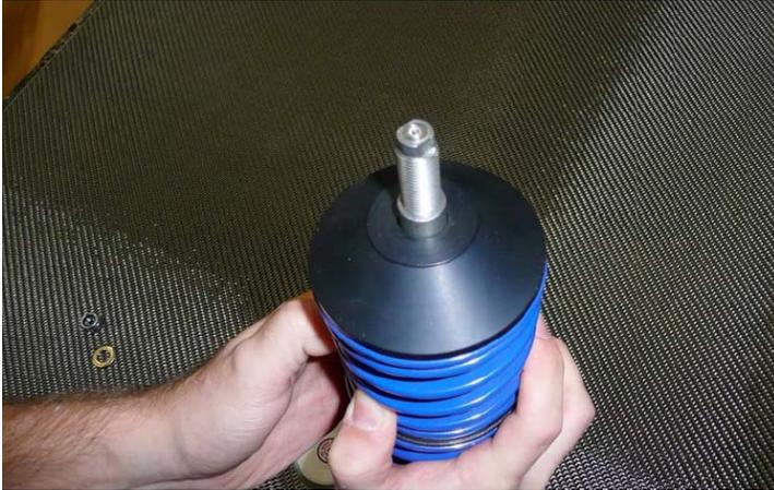
7) Install OEM Subaru conical washer.
