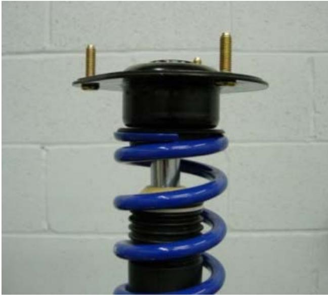
9) Thread the top nut onto the shaft of the damper and torque to 44 ft. lbs
