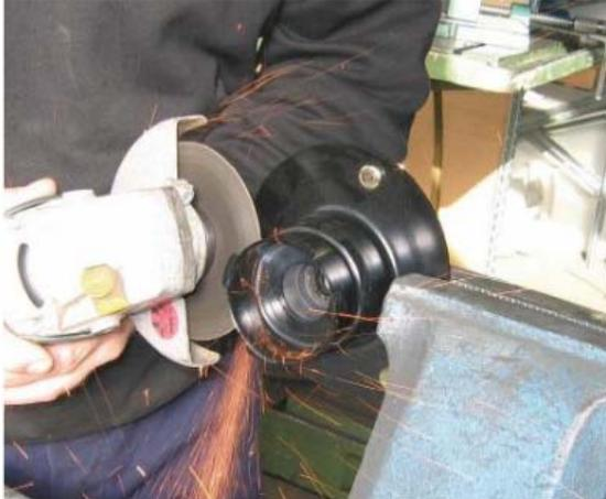
4) After the cut is complete, use a sanding disc to smooth out and flatten the cut. Be sure to remove any peaks or sharp edges.
