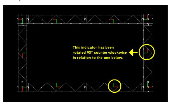
When the 90° corner block is used, the "running direction" of the truss changes. As such, the next truss piece is now rotated as shown by its indicator. This continues all the way around this rectangular truss structure until we connect back to the bottom left corner.
