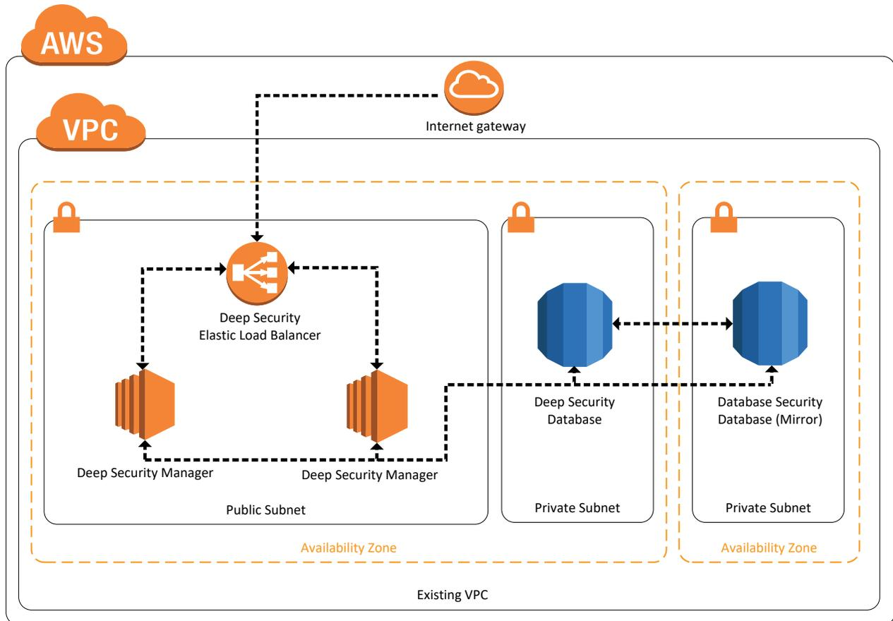
**Figure 1: Trend Micro Deep Security Architecture on AWS**
