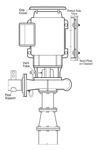
Providing proper procedures are followed, the Berkeley Type "B" Close-Coupled Electric Motor Drive End-Suction Centrifugal Pump may be mounted in a vertical position. The following are considerations that must be made:
