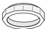
Pos. 104 Rotating Seal Face (The tapered face should point outward/upward through the driver 111 and press against the O-ring 107).
