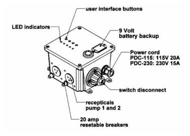
PDC-series controllers feature a programmed 6 hour run limiter for pump protection. If the alarm float remains closed (up position) for 6 hours but the primary float switch is open (down position) the alarm light will flash and the pump is turned off. This feature prevents the pump from running indefinitely and protects against run-dry situations.
