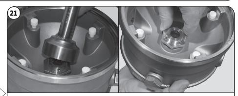
Flip the Pump Head Cover over to remove Shaft Seal (Pos. 105b). Using the specialty Tubular Box Spanner (00SV2107) or 41 mm Deep Socket, loosen and unscrew the Shaft Seal.
