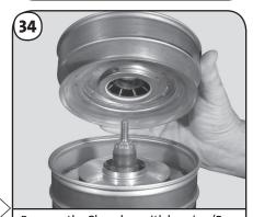
Remove the Chamber with bearing (Pos. 4a) or Chamber (Pos. 4). If it is stuck to the rest of the stack, pry it loose by inserting a screwdriver between the chambers.
