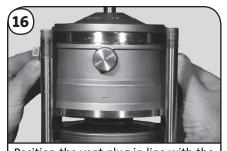
Position the vent plug in line with the vent sticker and flat surface of the sleeve flange. Lower the completed Cool-Top® Pump Head Assembly (Pos. 77a) over the Shaft and seat on the Sleeve (Pos. 55). If it does not freely seat onto the Sleeve, STOP. Remove the Pump Head and turn over. Remove sleeve O-ring and stretch. Replace and reinstall the Pump Head onto Shaft and Sleeve. Skip to step 22.
