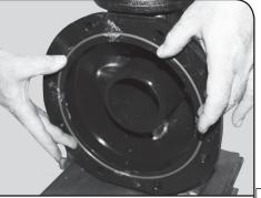
If this was not done earlier, remove the old O-ring and clean the groove. Next, in four equally spaced areas, place a liberal amount of Dow Corning 111 or Rocol onto the machined groove of the Suction/Discharge Base (Pos. 6). Fit the O-ring (Pos. 72a) into the groove, ensuring it is fully seated and does not move out of position.
