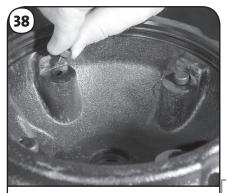
Remove the four Stack Compression Springs (Pos. 60) from the Motor Stool (Pos. 2) or Pump Head (Pos. 77 or 77a).
