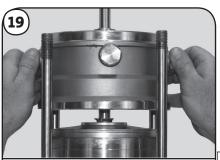
Position the vent plug in line with the vent sticker and flat surface of the sleeve flange. Lower the completed Pump Head Assembly (Pos. 77a) over the shaft and seat on the Sleeve (Pos. 55). If it does not freely seat onto the sleeve...**STOP**. Remove the pump head and turn over. Remove sleeve O-ring and stretch. Replace and reinstall the pump head onto shaft and sleeve.
