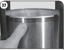
If the unit leaked around the Sleeve (Pos. 55), removal of the Sleeve may be required. Grip Staybolts (Pos. 26) diagonally. Using your thumbs, press against the Sleeve to release it from the Sleeve Flange Housing (Pos. 55b). Lift off sleeve. (Rocking or light upward blows with a rubber mallet may be required.)
