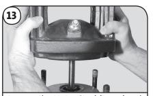
Remove the Motor Stool (Pos. 2) and Pump Head (Pos. 77) on N models. (Light upward blows with a rubber mallet may be required.)
