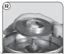
Lift the Impeller (Pos. 49a) off the shaft. If it comes off freely, proceed to step 34. If it is stuck and cannot be removed by hand, proceed to step 33.
