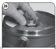
Finish removal of Shaft Seal (Pos. 105b) from Pump Head Cover (Pos. 77a). Flip the Pump Head Cover over and go to step 27.
