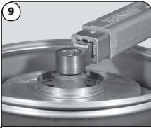
Lubricate the threaded end of the shaft with Gardolube (00SV9995). Thread the Lock Nut (Pos. 67) onto the shaft and torque to 16.3 ft.-lbs./22 Nm. Use 13 mm Socket (00SV0091), Ratchet (00SV0295), and Torque Wrench, (00SV0269).
