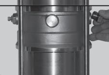
Loosen and remove the plug to allow access to Shaft Seal securing screw. Insert a 2.5 mm allen wrench to loosen (approximately 1/2 to 1 turn) the three Set Screws (Pos. 113) of the Inboard Seal (Pos. 105b).
