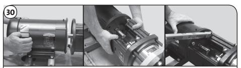
Slide the motor assembly toward the Motor Stool and/or Spacer (Pos. 1), then install and tighten Motor Bolts (Pos. 28) diagonally to the proper torque.
