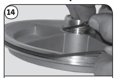
Place O-rings (Pos. 109a & 37c) onto the Disk Plate (Pos. 79a). Do not roll the O-rings; they should be stretched over and released into place to prevent cutting the material during installation into the housing. Lubricate the O-ring with Dow Corning 111 or Rocol (00RM2924) or spray soapy solution onto O-rings and housing.
