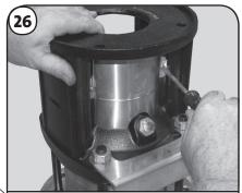
Place the first Coupling Guard with the support bracket. Install screws (pos. 7a) using a torque screwdriver with a slotted or Torx® tip T20, torque to 1.5 ft.-lbs./2 Nm. The cartridge assembly is now ready to take back to where the suction discharge volute is located.
