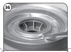
To remove Seal Ring (Pos. 45), insert a slotted screwdriver in relief slot of Seal Ring Retainer (Pos. 65) and twist or use Puller (00SV0239).
