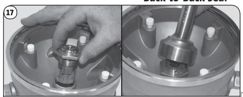
Insert Inboard Seal (Pos. 105b) into the bottom side of the prepped Pump Head Cover (Pos. 77a). Using the specialty Tubular Box Spanner (00SV2107), or a 41 mm Deep Socket, tighten/torque seal the 26 ft.-lbs./35Nm.
