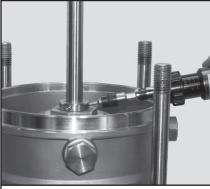
Push down on the coller area of the Seal, then lift Shaft to create a clearance of 123 mm from the top of the Shaft (Pos. 51) to the top of the Shaft Seal. Tighten the three 2.5 mm set screws to 2 ft.lbs./2.5 Nm. Proceed to step 22.
