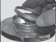
Wear Rings (Pos. 49c) can be removed on CR-H, CRN-H 15 and 20 models. Impellers (Pos. 49a) use Puller (00SV0239) and Support (00SV0043) to work Wear Ring off of impeller.
