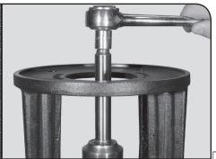
Pushing down on Shaft Seal collar (do not push down on Hex Nut), lower the new Shaft Seal (Pos. 105) over the Shaft. Use the specialty Tubular Spanner (00SV2107), a 41 mm Open Ring Spanner (00SV2101), or a 41 mm Deep Socket to tighten to 26 ft.-lbs./35 Nm.
