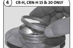
Press new Wear Ring (Pos. 49c) onto Impeller (Pos. 49a). Use new Impellers if eyelet of Impeller is worn.
