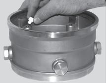
Remove Sleeve O-ring (Pos. 37) from the pump Head Cover (Pos. 77a). Then, remove the PTFE Stack Compression Springs (Pos. 60a) from the Pump Head Cover.
