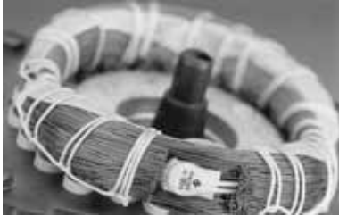
Fig. 43 Thermal switch incorporated in windings
