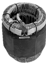
Fig. 39 Mains-operated motor with anti-condensation heater
