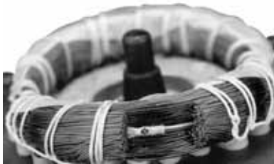
Fig. 41 PTC sensor incorporated in windings
