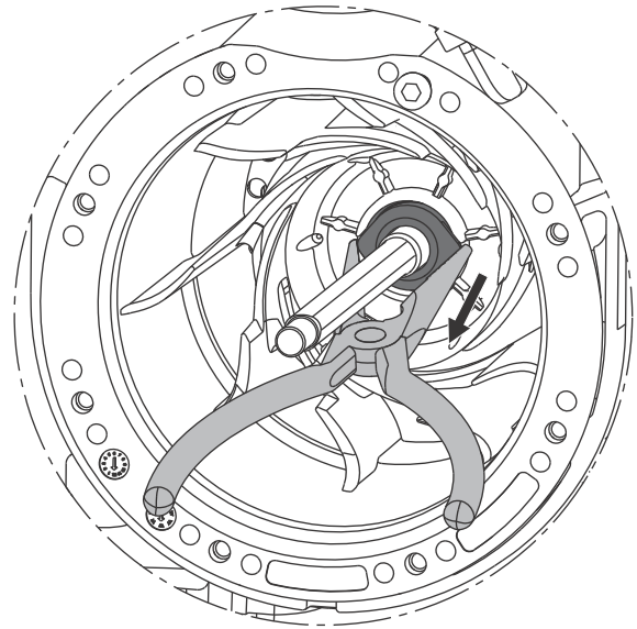
Fig. 12 Removing the stationary shaft seal
