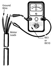
by 0.61 to determine the actual resistance of aluminum cable.
