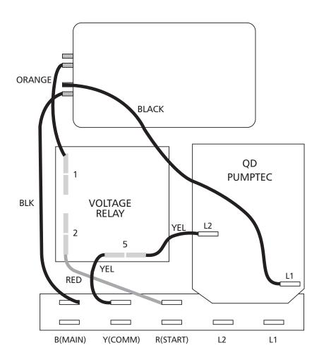
CENTRIPRO CONTROL BOX WITH PUMPTEC INSTALLED
