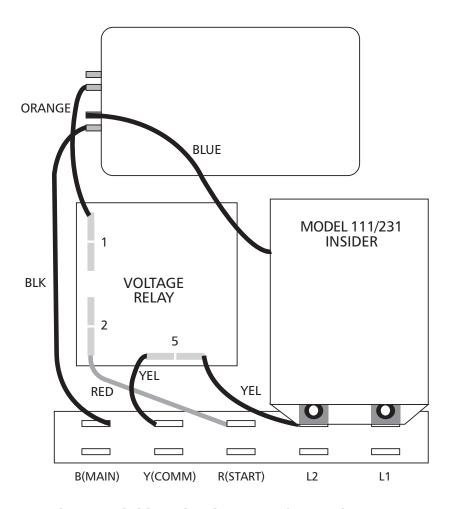
CENTRIPRO CONTROL BOX WITH INSIDER INSTALLED
