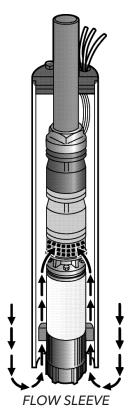
MINIMUM FLOW RATES FOR PROPER MOTOR COOLING
