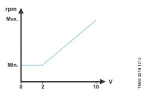
Fig. 32 External setpoint function, 0-10 V
