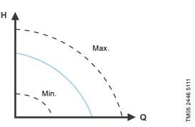
Fig. 20 Max. and min. curves
