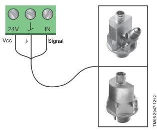
Fig. 17 Examples of external sensors
