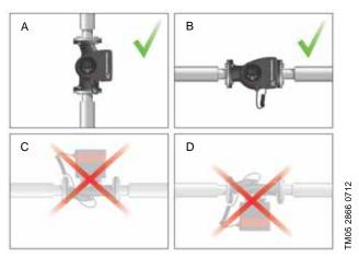
Fig. 7 Pump installed with horizontal motor shaft
