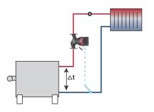
Fig. 27 Differential temperature
