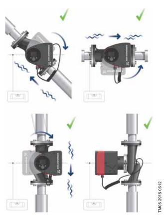
Fig. 8 Pump with control box in horizontal position
