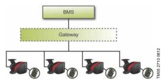
Fig. 35 Building management system (BMS) with four pumps connected in parallel
