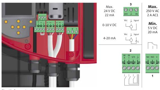
Fig. 12 Connection diagram
