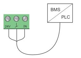
Fig. 18 Examples of external signal for the control via BMS/PLC
