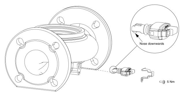
Fig. 34 Correct position of sensor
