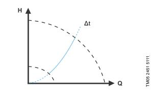
Fig. 26 Differential temperature
