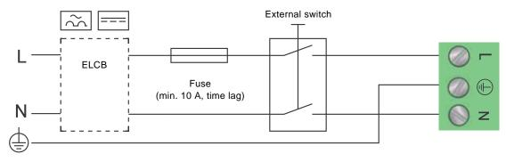
Fig. 11 Example of typical connection, 1 x 230 V  $\pm$  10 %, 50/60 Hz
