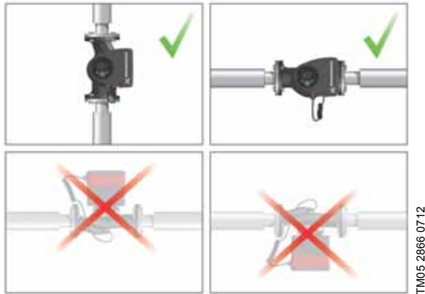
Fig. 10 Installation positions
