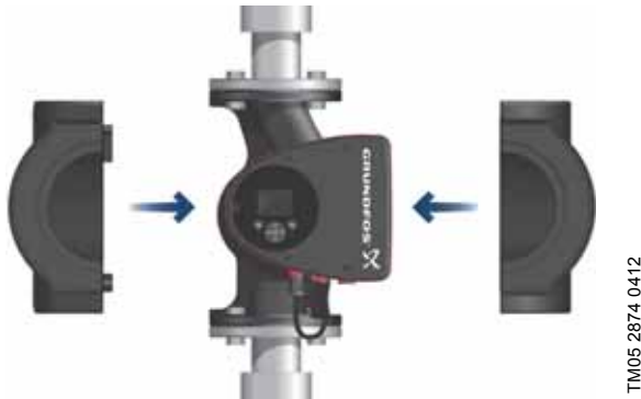
Fig. 57 Fitting the insulating shells to a MAGNA3 pump
