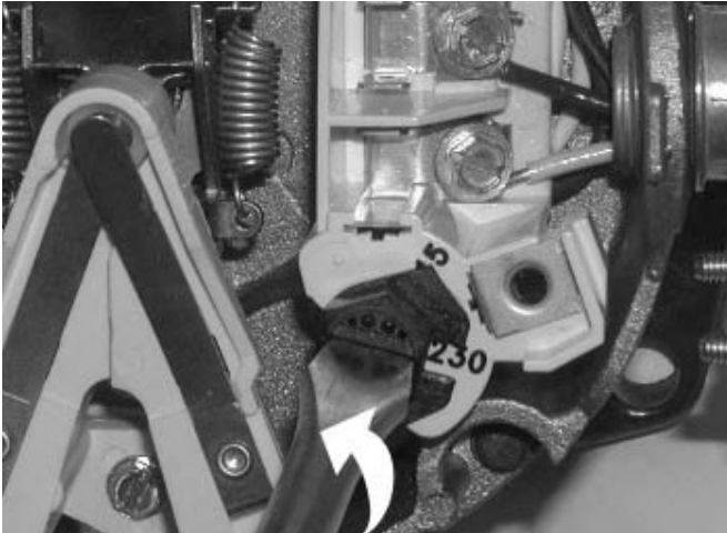
Figure 5: Changing the Voltage Setting.
