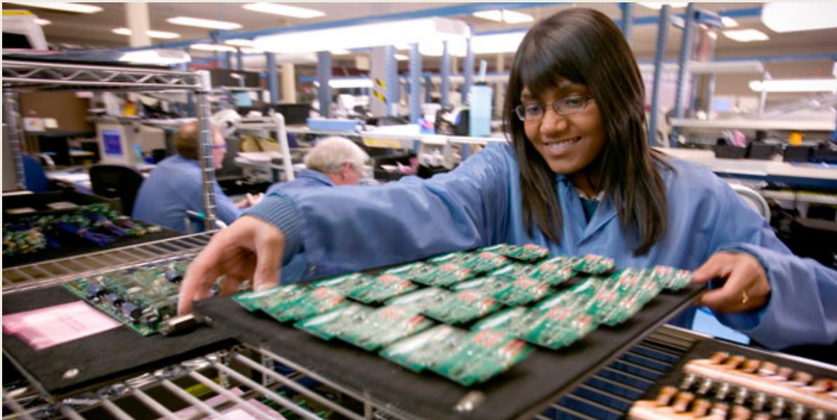
*As an intern at Garmin AT, electrical and computer engineering student Shannon Mark tests a tray of circuit boards destined for remote-control devices for aircraft radios. (Photo courtesy of Garmin AT, Inc.)*
