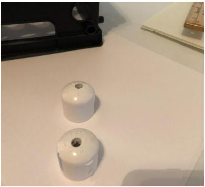
Take a ½" PVC cap and drill a hole I the middle. Attach the rope to the cap and secure it with duct tape.
