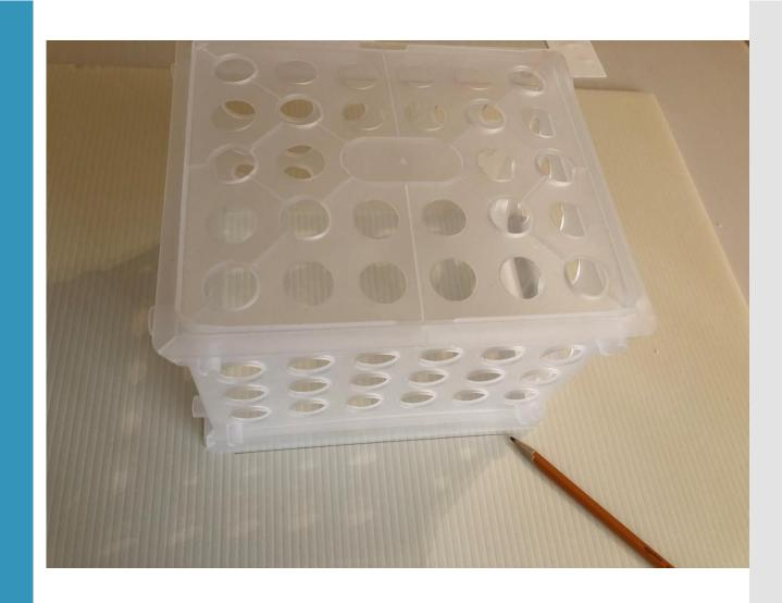
Remove the crate measure approximately 1/2" and draw a second mark. It should be one mark inside the crate and the other outside.
