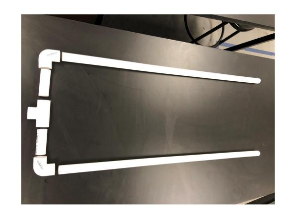
Attach each end of the PVC Tee to each end of the elbows and join the pieces.
