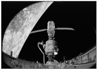
The STS-88 crew uses the robotic arm to mate the Unity module to the Zarya module.
