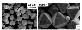
Zeolite Crystals on the left were grown on earth. The ones on the right were grown in microgravity.
